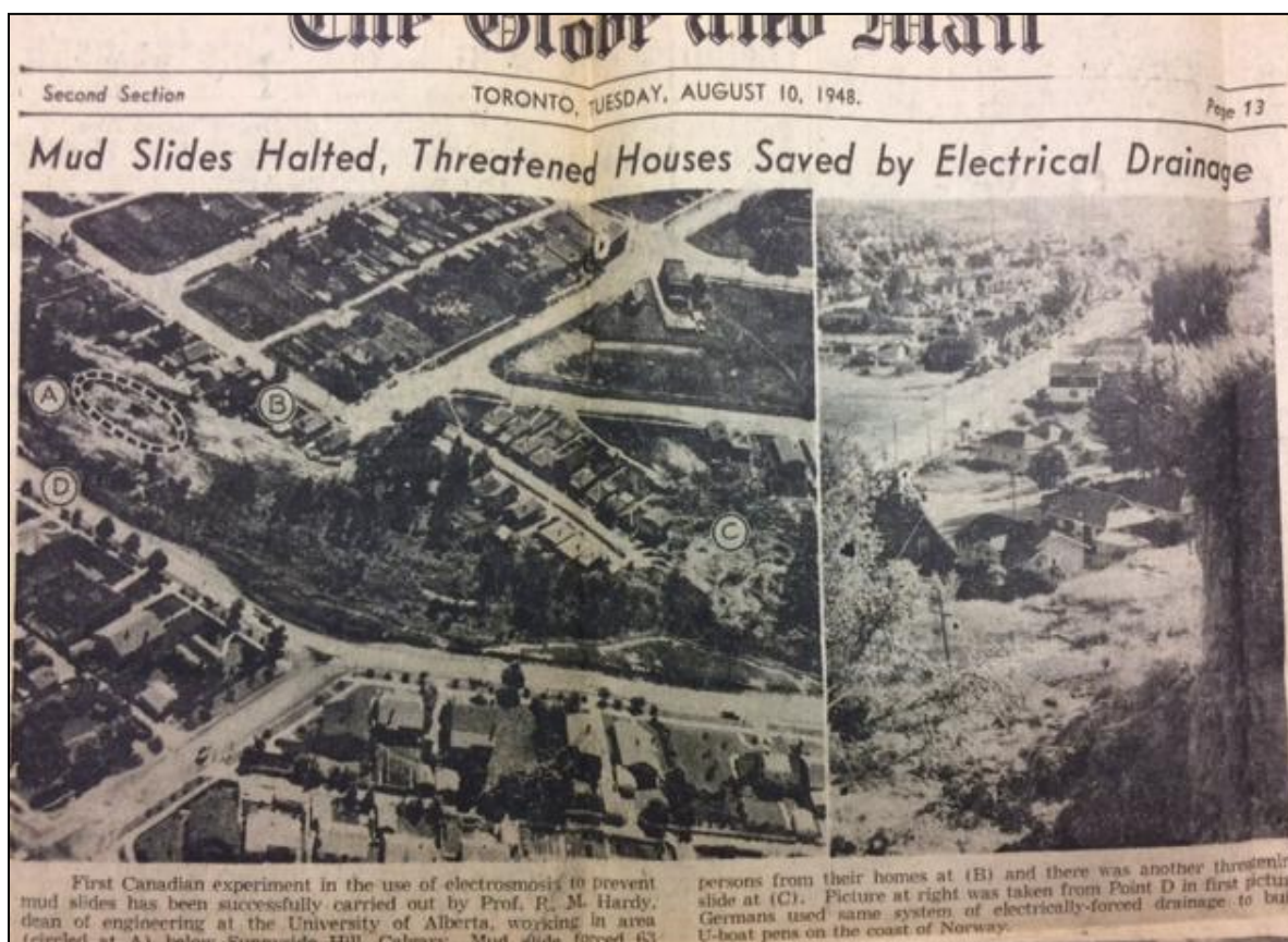
Figure D5. Calgary made the second section front page of The Globe and Mail in August 1948. The photo caption announces the use of electromosis to try to dry the mud flow (first in Canada). It was not effective. Only three years after WW II, an analogy is made to U-boat pens in Norway to hook the reader.
