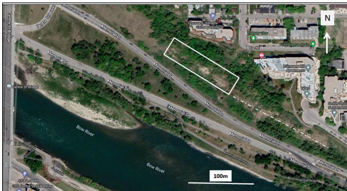
Figure 15. Satellite photo of East Crescent Heights Escarpment. The dashed line shows where a band of bedrock is exposed about 10 metres vertically above the base of slope. The white rectangle encloses an area of slope modification, perhaps indicative of excavation of a quarry bench.
