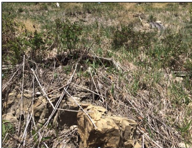
Figure 18. Photo of yellow, blocky sandstone at west end of outcrop band. Sandstone bed is about 0.2 metres thick.
