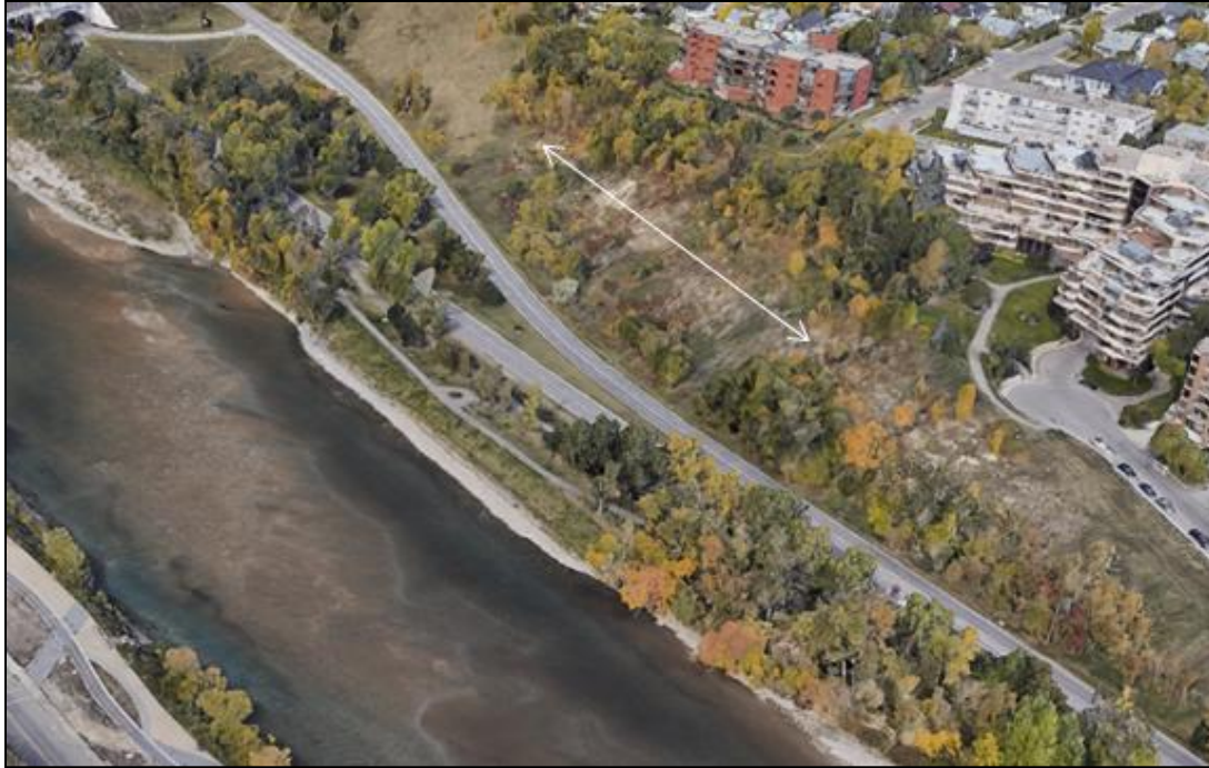
Figure 26. Satellite Image of slope above projected sandstone outcrop. The slope has been extensively reworked with flat spots and bowls on slope above the top bedrock elevation. This is consistent with overburden removal in the building of a quarry bench back into the hill. The arrow shows the extent of the slope reworking.
