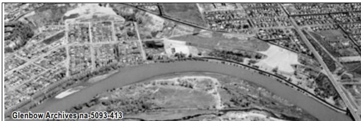
Figure D12. Glenbow Archives 1967 aerial photo of McHugh Bluff. The remnants of the 1958 slide are still obvious as white coloured area on bluff. As is the area of the 1932 slide - you can see where it covered the low angle tramline path that ran up to Centre Street.
